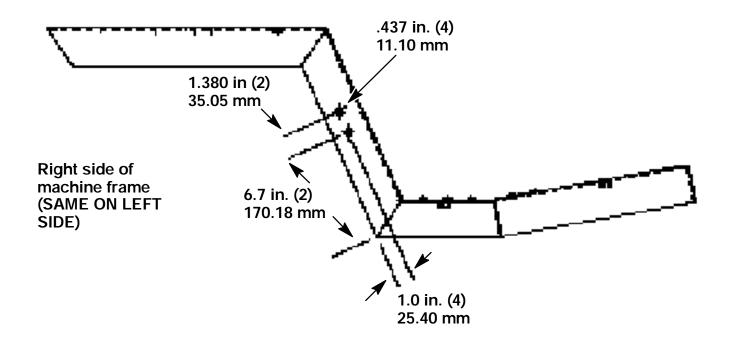
FIG. 1 - Bracket Mount Hole Location Drawing
